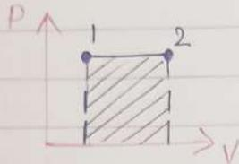
$$W_{1-2} = \int_1^2 P dV = P(V_2 - V_1)$$
