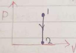
$$W_{1-2} = P dV = P(V_2 - V_1)$$
